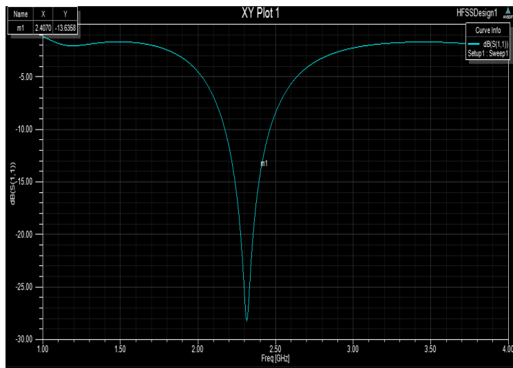
Fig 4. Simulated reflection coefficient versus frequency
